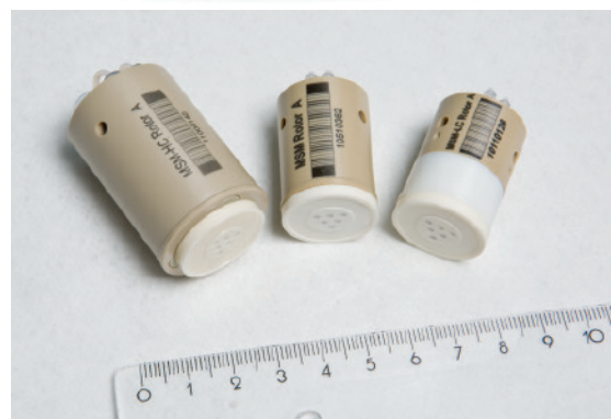
All three suppressor rotors – MSM-HC, MSM, and MSM-LC – have the same design and vary solely in terms of their capacity.
