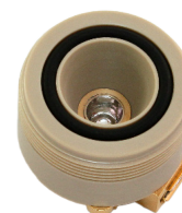
Sample container with PEEK cover
