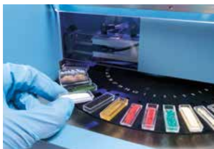
Sample boat is placed into the autosampler
