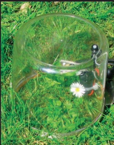
The CPY-2 is designed for closed system measurement of canopy CO 2 flux.
