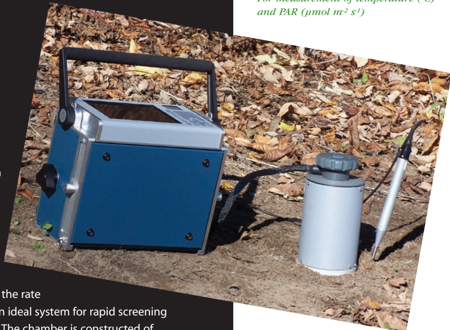
The CIRAS-2 shown with the SRC-1 Soil Respiration Chamber and STP-1 Soil Temperature Probe.
