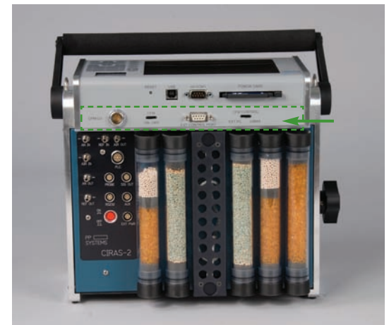
The CIRAS-2 shown above with integral Chlorophyll Fluorescence Module (CFM) signal conditioning interface.
