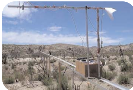
The UniSpec-DC mounted on a tram based system for unattended, automated optical sampling along a transect
