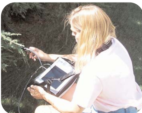
Measurement of leaf level reflectance in the field with UniSpec-SC, bifurcated fiberoptic and leaf clip
