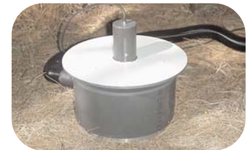
CFX-2 Soil Respiration Chamber (Open)
