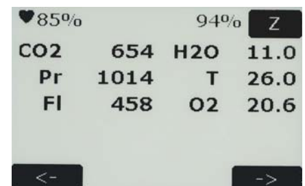
Monitor multiple sensors including CO 2 , H 2 O and O 2 from one display
