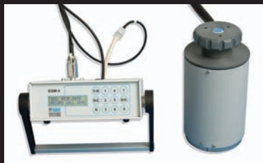
Soil CO 2 Efflux with EGM-4
