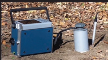
Soil CO 2 Efflux with CIRAS-2
