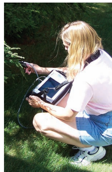
Leaf reflectance measurement in the field with UniSpec-SC
