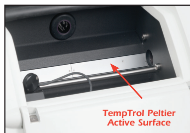
TempTrol heating and cooling Peltier transfer surface
