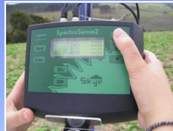
SpectroSense2+ with GPS for mapping
