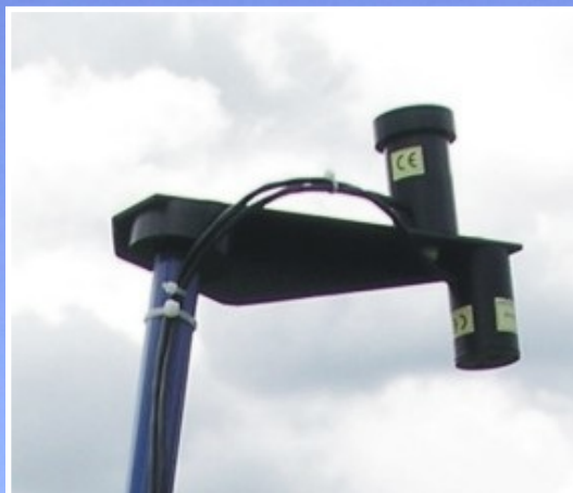
Sensors mounted for measuring incident & reflected light
