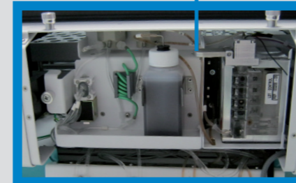
ISE module for pH, conductivity and redox analysis
