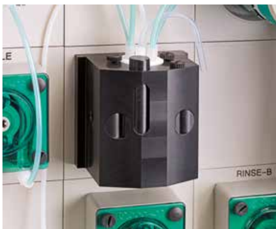
Cuvette module for photometric measurements
