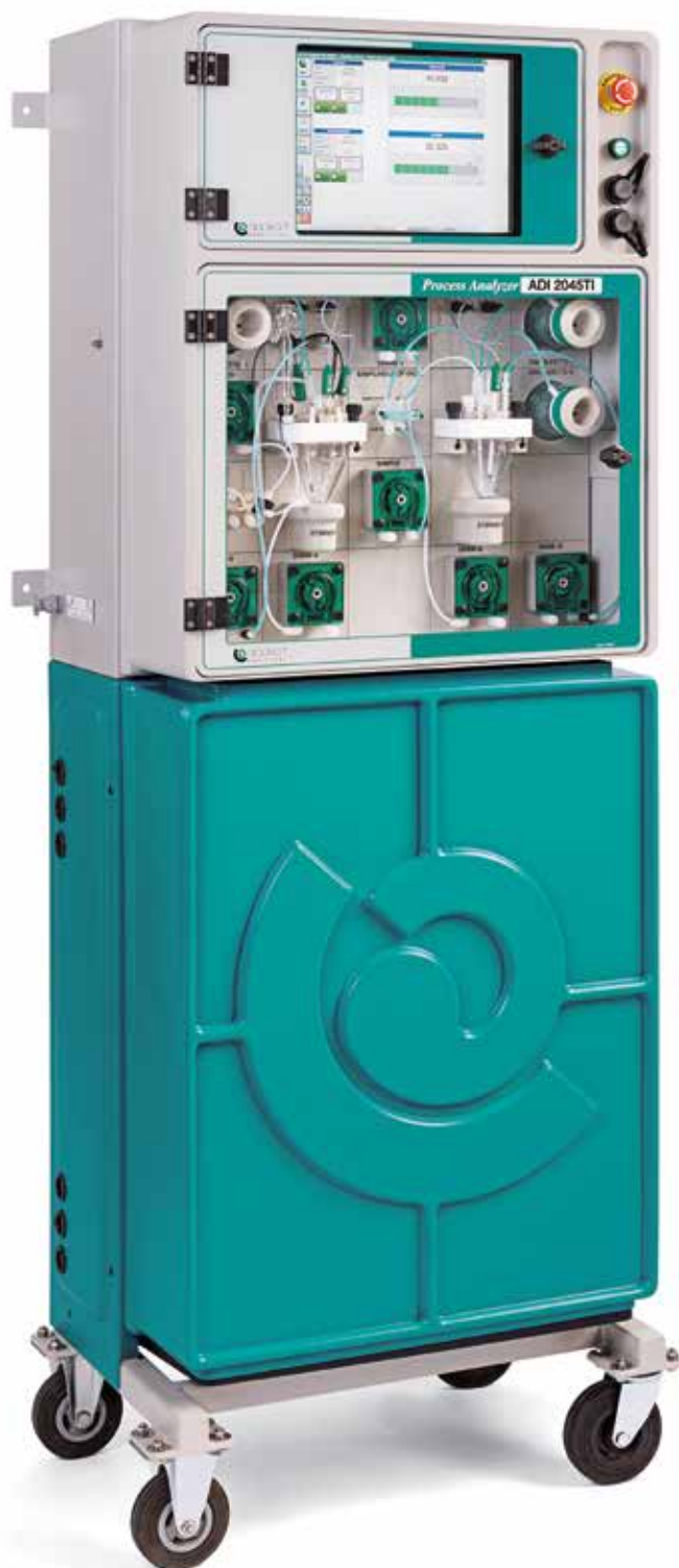
ADI 2045TI Process Analyzer for online monitoring of various parameters
