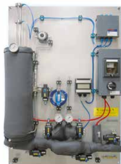
Sampling system for determining the water content in hydrocarbons
