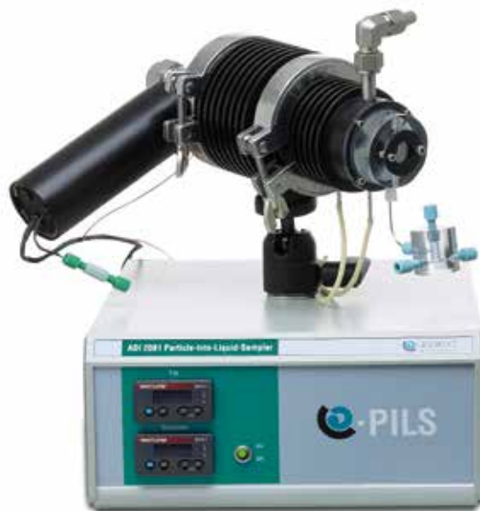
The Particle Into Liquid Sampler. PILS coupled with IC and VA can be used to measure the ionic substances of the aerosols.
