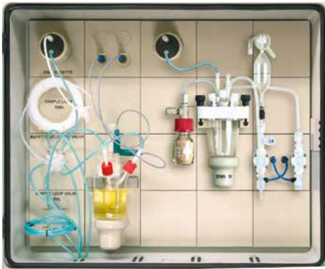
ADI 2045Ti Process Analyzer for coulometric determination of water content according to Karl Fischer
