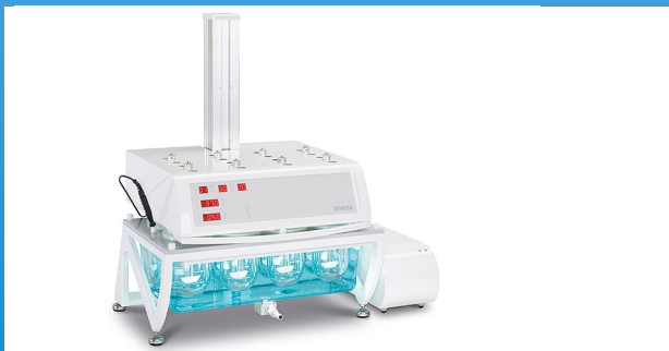
DT 728 in Low-Head mode to minimise evaporation
