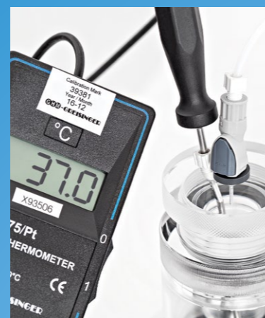
Special temperature calibration head.
