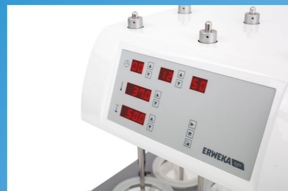
LED display and symbol keypad for easy control
