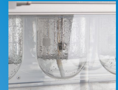
Automatic cleaning and result checks of the cleaning process (SST).
